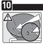
▲ Finger Tighten Only. Do not fully tighten any of the screws before both the table and bowl assembly have been installed.
